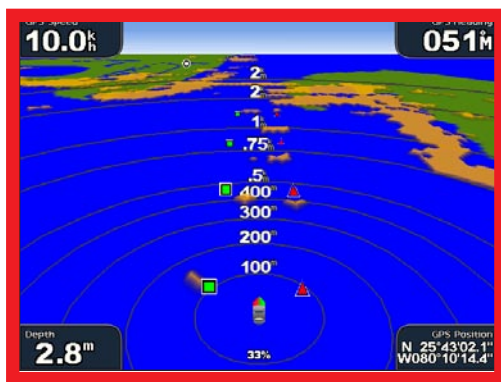
Mariner’s Eye With Radar Information
